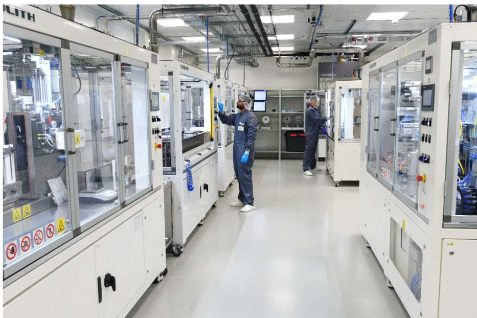
Fig. 3: Semi-automated production line for industrial-scale pouch cells in the cleanroom at Fraunhofer ISE's Center for Electrical Energy Storage. © Fraunhofer ISE
