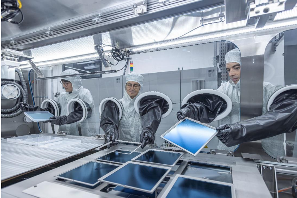
Fig. 2 Pero-Si-SCALE transfers cell designs from the laboratory to industrial cell formats up to a wafer size of 210 by 210 square millimeters. © Fraunhofer ISE / Photo: Michael Spiegelhalter
