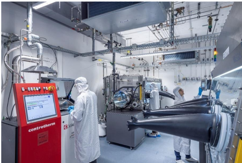
Fig. 3 For the manufacturing process of perovskite-silicon tandem solar cells, Fraunhofer ISE focuses on the so-called “hybrid route,” a combination of vacuum and wet chemical processes. © Fraunhofer ISE / Photo: Michael Spiegelhalter
