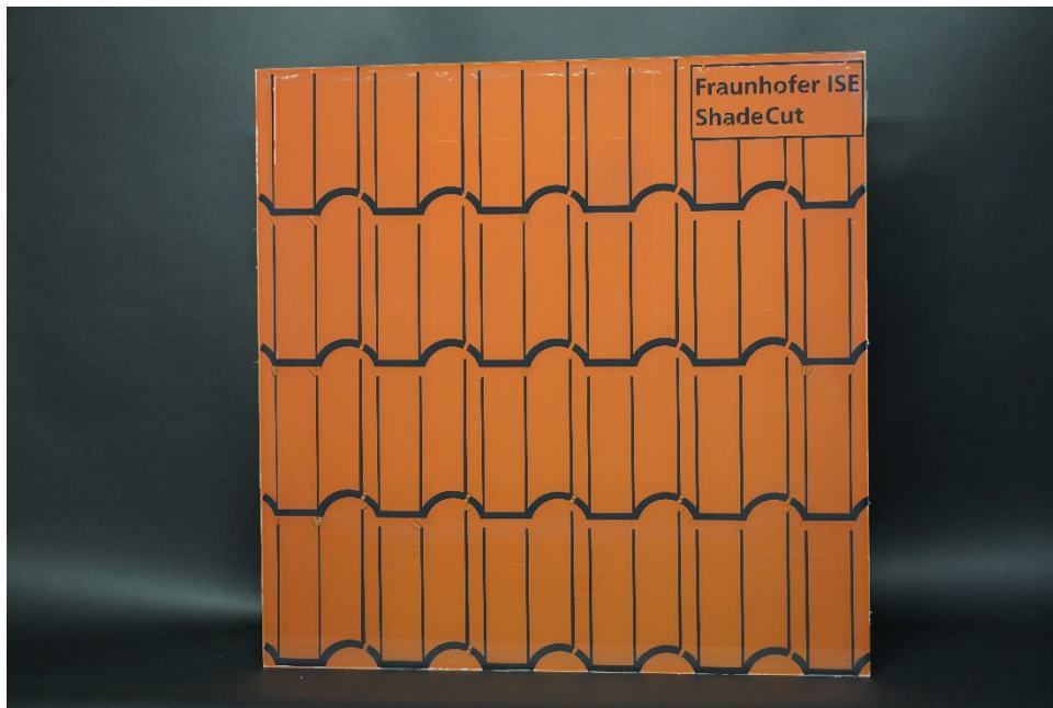
Fig.1 The foil cutting patterns can be used, for example, to imitate roof tiles without significantly impairing the efficiency of the PV module. © Fraunhofer ISE / Photo: Marco Ernst
