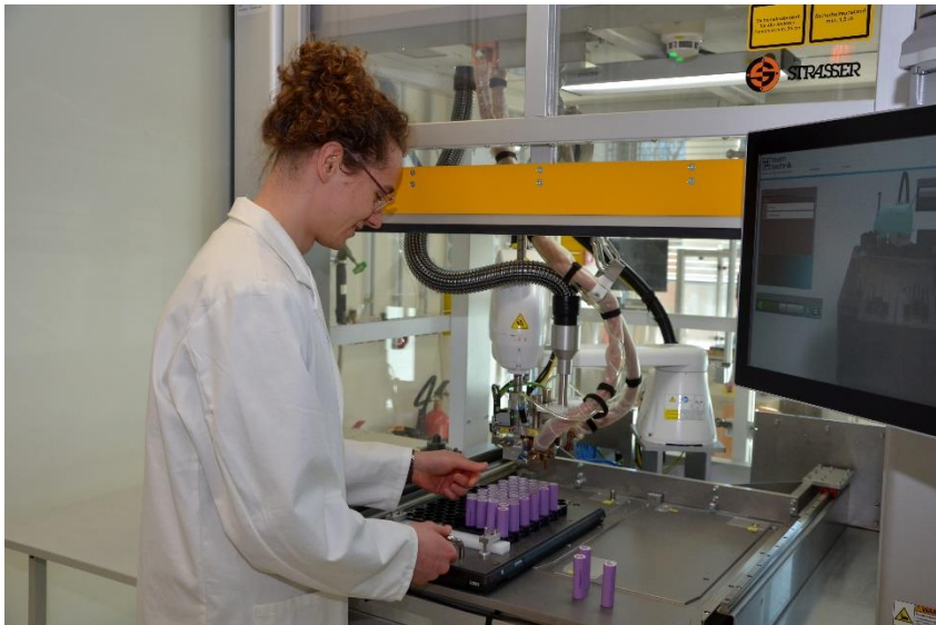
Project Manager Christian Schiller at a projection welding machine where battery cells are connected using copper connectors. © Fraunhofer ISE / Photo: Felix Thurn
