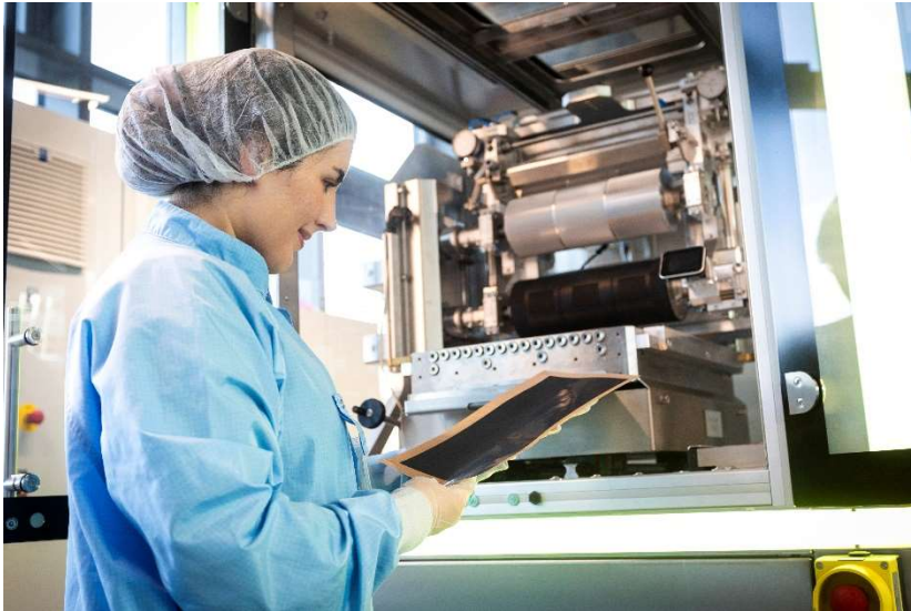
The pilot line offers various printing and coating processes for the production of catalyst layers. © Fraunhofer ISE/Dirk Mahler
