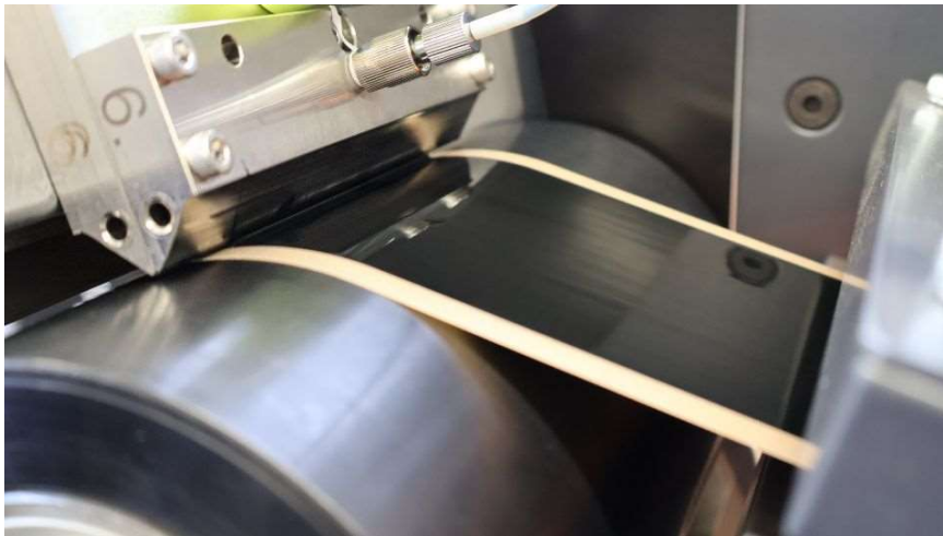
Catalyst ink is continuously applied on a transfer foil via a slot die coating. © Fraunhofer ISE
