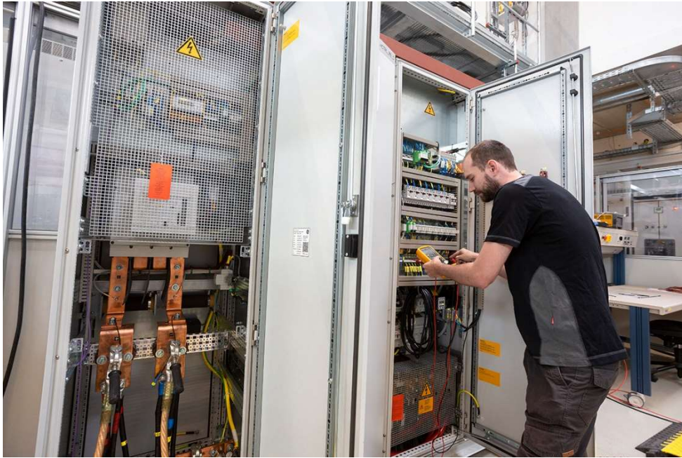
Preparation of a grid-forming inverter for measurement in Fraunhofer ISE's multi-megawatt lab. © Fraunhofer ISE
