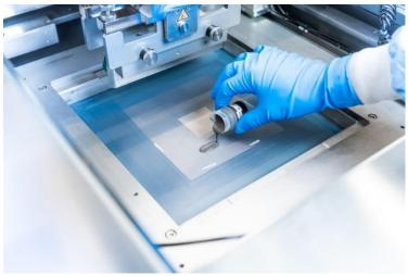
A paste consisting of titanium powder, solvent and additives is applied to the pressure screen. The paste is then applied through the screen as a thin microporous layer onto a titanium fibre substrate using a squeegee. © Fraunhofer ISE/Joscha Feuerstein
