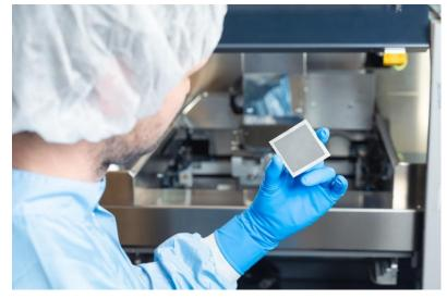
Final microporous layer on a titanium fibre substrate after the screen printing process. In a subsequent step, the two layers are sintered. The microporous layer with a reduced surface roughness allows an optimized interface to the catalyst layer. As a result, the catalyst loading with iridium can be reduced and thinner membranes are possible. © Fraunhofer ISE/Joscha Feuerstein
