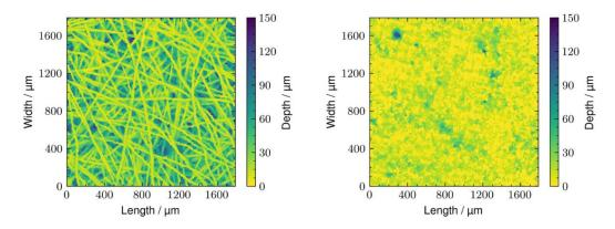
The laser scanning microscopy image shows the significant reduction in surface roughness. © Fraunhofer ISE
