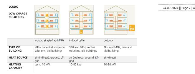
Fields of application in the LCR290 project: floor heating, central heating in the basement, high-performance heat pumps for outdoor installation (LT-grid: low-temperature heating network). © Fraunhofer ISE
