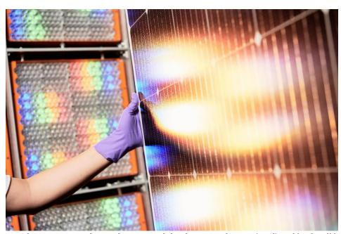
In order to measure the tandem PV module, the research team irradiated both cell layers in a special solar simulator developed specifically for this purpose. © Fraunhofer ISE / photo: Bernd Schumacher
