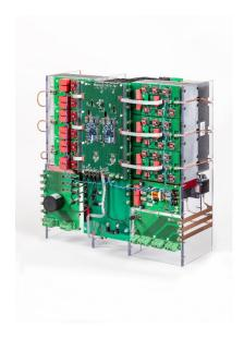
The inverter developed by Fraunhofer ISE enables the transition of PV from low voltage to medium voltage. © Fraunhofer ISE
