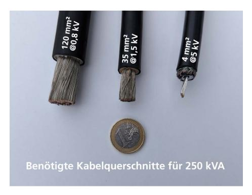
Higher voltage reduces the cable cross section. © Fraunhofer ISE
