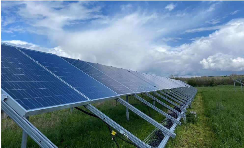
PV module test stand at the new Outdoor Performance Test Field, where Fraunhofer ISE will be testing various solar technologies. © Fraunhofer ISE / Photo: Sophia Bächle
