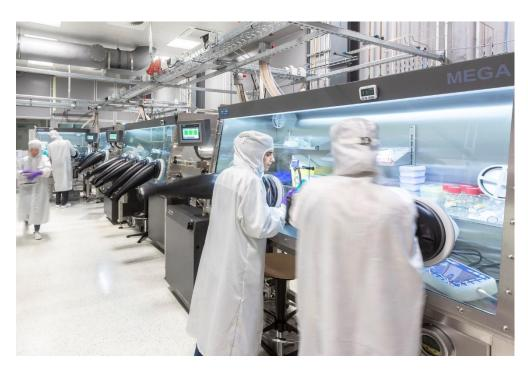
Processing perovskite-silicon tandem solar cells at Fraunhofer ISE. The lab infrastructure comprises evap-oration chambers for perovskite absorbers, selective contacts and metals, and the atomic layer deposi-tion of metal oxides under an inert gas atmosphere. © Fraunhofer ISE
