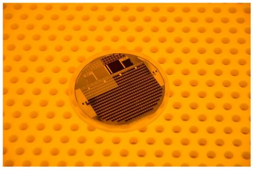
Thanks to improved antireflection layers, the efficiency of the best four-junction solar cell to date improved from 46.1 to 47.6 percent. © Fraunhofer ISE
