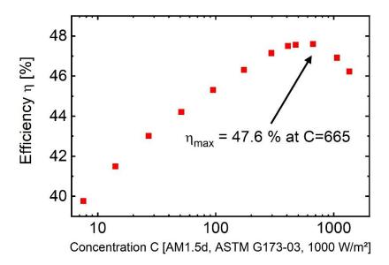
The efficiency of the new four-junction solar cell increases with concentration up to 665 suns, reaching a value of 47.6 percent conversion efficiency for the first time. © Fraunhofer ISE
