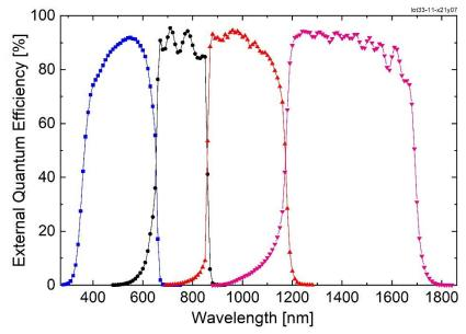
Quantum efficiency of the new four-junction solar cell. The top sub-cell made of GalnP absorbs short-wave sunlight in the visible spectral range. Infrared light is converted in the sub-cells underneath which are made of AlGaAs, GalnAsP and GalnAs respectively. © Fraunhofer ISE
