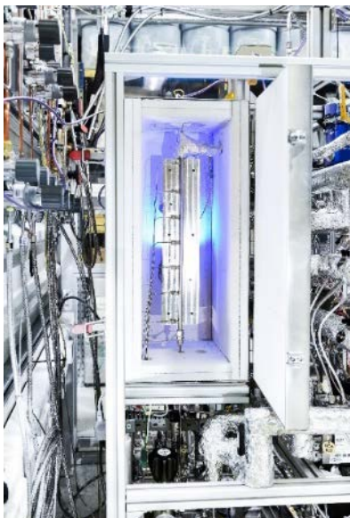
Front view of the reactor with open furnace door. The compact and mobile system is designed for use on location. © Fraunhofer ISE
