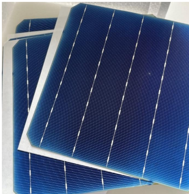
PERC solar cells made of 100 % recycled silicon with an efficiency of 19.7 percent. © Fraunhofer ISE
