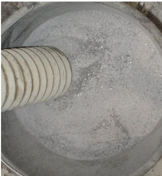
By-products of the treatment process at Reiling GmbH, from which the solar cell fragments are separated and collected. © Fraunhofer ISE
