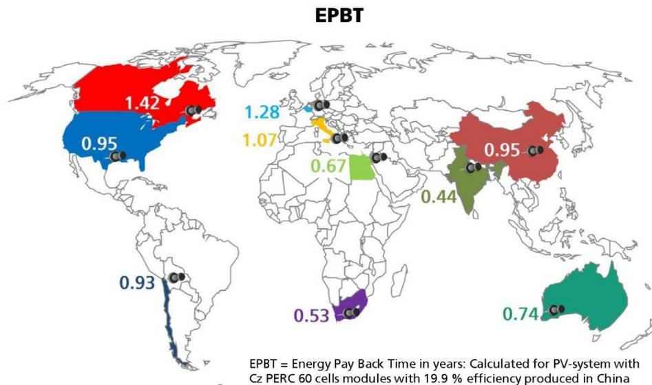
The energy payback time, or EPBT, for rooftop systems with silicon PV modules of 19.9 percent efficiency, manufactured in China, is one year and one to three months in Europe. Data: Lorenz Friedrich, Fraunhofer ISE. Graph: PSE 2020. ©Fraunhofer ISE
