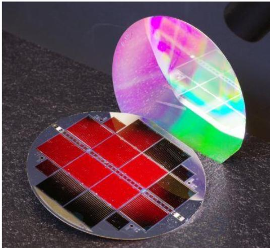
The new III-V//Si tandem solar cell with 35.9 % efficiency. The top subcell glows red, which is a sign of outstanding material quality. The nanostructured back side of the cell shimmers in rainbow colors.
