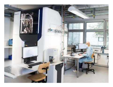
The NAP-XPS system of Fraunhofer ISE provides multi measurement performance for material characterization. © Fraunhofer ISE
