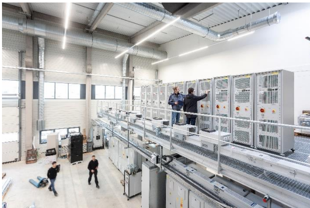
In the Multi-Megawatt Lab, components and systems are tested up to 10 MVA. ©Fraunhofer ISE/Dirk Mahler
