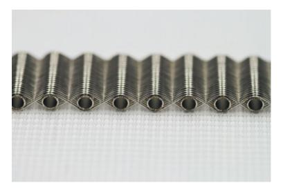
The structure is made of stainless steel and is thus suitable for corrosive PCMs. ©Fraunhofer ISE
