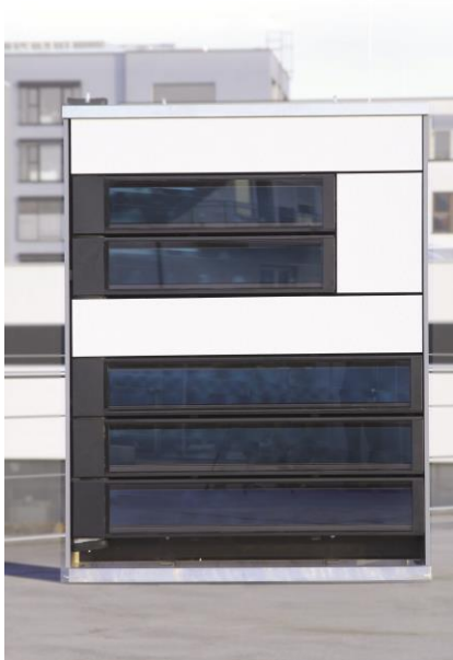
The strip collectors can be produced in a variety of different lengths. ©Fraunhofer ISE
