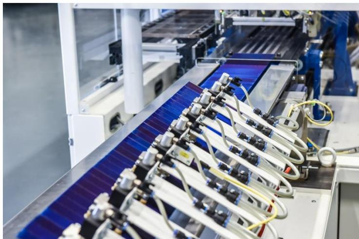
Pilot process to apply an electrically conductive adhesive to shingled cells carried out on the industrial stringer in the Module-TEC of Fraunhofer ISE. ©Fraunhofer ISE
