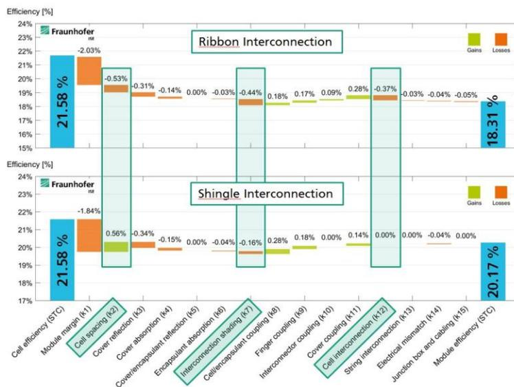
Screen shot of a waterfall diagram from the software package SmartCalc.CTM of Fraunhofer ISE, where the efficiency gains and losses of a single cell module to a module with conventional cell interconnections are compared. ©Fraunhofer ISE
