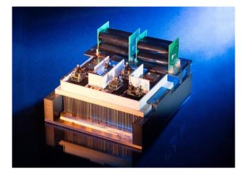
Single-phase 20 kV power stack with 15 kV silicon carbide power MOSFETs, drivers and part of the DC link capacitors. ©Fraunhofer ISE
