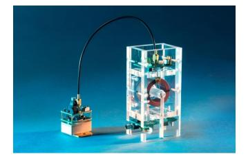
15 kV silicon carbide MOSFET with mounted gate driver and galvanically isolated supply. ©Fraunhofer ISE
