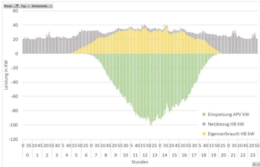
In summer, the electricity demand of the farm was almost completely covered by the PV array. © BayWa r.e. renewable energy / Fraunhofer ISE
