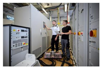
In the longstanding TestLab Power Electronics of Fraunhofer ISE, power converters of all types are tested and developed up to the range of 1 MW. With the new lab facility in Freiburg, the solar research institute is expanding its services to include the multi-megawatt range. ©Fraunhofer ISE
