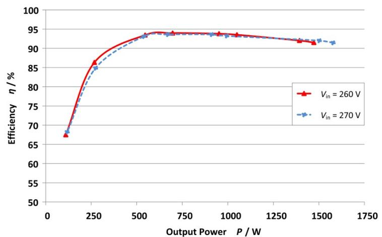
Efficiency measurements for different power outputs of the highly compact DC/DC converter developed at Fraunhofer ISE for aviation applications. ( $V_{out} = 28$  VDC,  $f_{sw} = 1.8$ -2.5 MHz). The maximum efficiency is 94.5 %. ©Fraunhofer ISE
