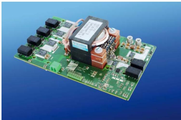
New materials enable high speed frequencies: Fraunhofer ISE develops resonant DC/DC converters with 2.5 MHz as demonstrator for aeronautical applications. ©Fraunhofer ISE
