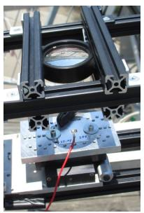
World record for concentrator photovoltaic technology: mini-module comprised of four-junction solar cells reached 43.4 percent efficiency. ©Fraunhofer ISE
