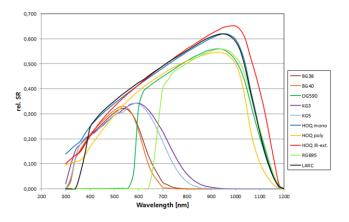
Spectral response (<u>Relative Spectral Response</u>) of various reference cells in comparison with the new type (HOQ IR ext.). ©Fraunhofer ISE
