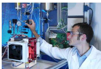
Test stand for water electrolyzers. ©Fraunhofer ISE
