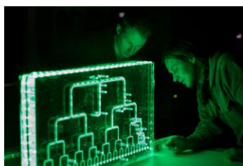
Measuring a distribution system for a refrigerant evaporator. ©Fraunhofer ISE
