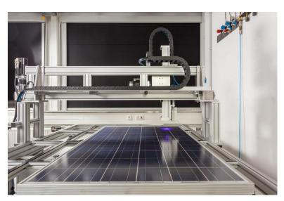
Multi-purpose table for characterizing PV modules and testing new, non-destructive measurement techniques – developed and used by Fraunhofer ISE. ©Fraunhofer ISE
