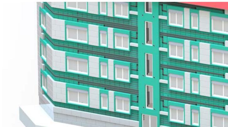
Model shows the wiring and pipes integrated in the façade of a demonstration building from the 1950s in Frankfurt, Germany.
