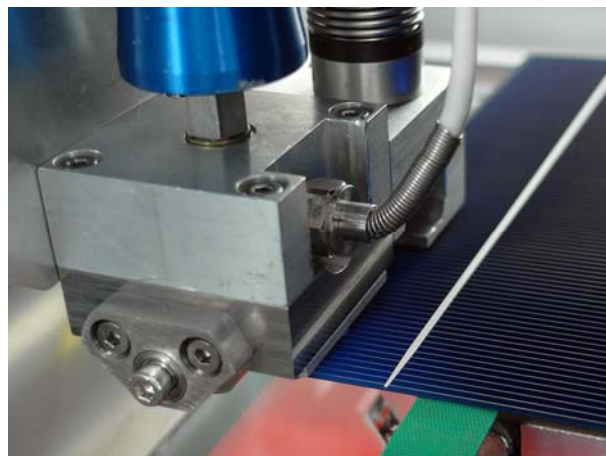
Fraunhofer ISE's newly developed automatic dispenser with ten nozzle printhead. ©Fraunhofer ISE
