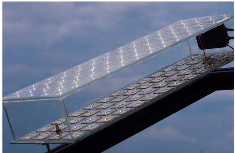
Newest FLATCON® concentrator module with an efficiency of 36.7 %.
