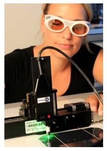
Researcher seated at the Raman spectrometer: Non-destructive investigation of polymer components in PV modules. @Fraunhofer ISE
