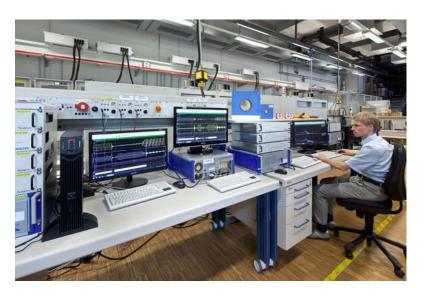
High-resolution measurement system for analyzing the power of solar parks in detail. The system enables synchronous data acquisition of the currents and voltages of several solar inverters which are locally distributed. ©Fraunhofer ISE
