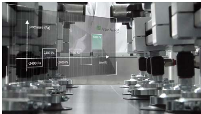
PV module in a mechanical stress test. ©Fraunhofer ISE
