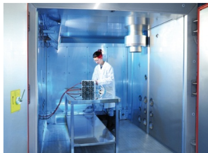
Walk-in climate chamber used for tests on fuel cell stacks and systems © Fraunhofer ISE
