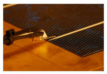
The accredited CalLab PV Cells at Fraunhofer ISE has been measuring solar cells for customers for many years. ©Fraunhofer ISE
