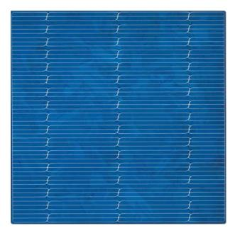
Multicrystalline MWT solar cell (156 x 156 mm²). The photo shows the developed contact structure. Through the tiniest holes, the connection to the back side of the solar cell is established.  $\[ \]$  Fraunhofer ISE
