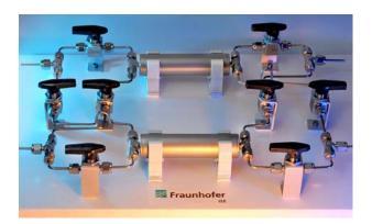
Model of pyrolysis system with two reactors. The ball valves are set so that pyrolysis takes place in only one reactor at a time, while the other reactor regenerates. The switching is controlled in such a way to produce a high concentration of hydrogen and a low concentration of carbon monoxide. ©Fraunhofer ISE
