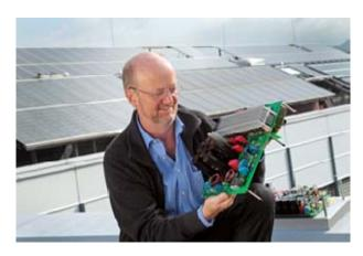
Dr. Heribert Schmidt, winner of the Fraunhofer Prize 2011, invented a new circuitry for the inverter. With the HERIC® technology, it was possible to achieve a world record for inverter efficiency of >99% at Fraunhofer ISE (©Dirk Mahler).
