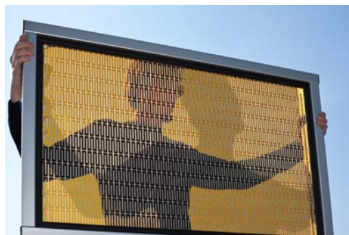
Prototype of a 60 x 100 cm 2 dye solar cell module manufactured at Fraunhofer ISE using a screen-printing process. ©Fraunhofer ISE
