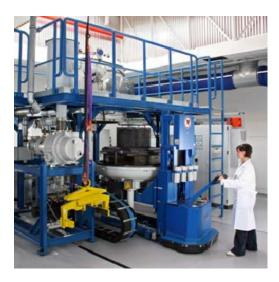
Crystallization unit for producing multicrystalline silicon blocks. @Fraunhofer ISE
