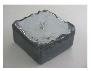
Multicrystalline silicon block (13kg) manufactured at SIMTEC Fraunhofer ISE using the Vertical Grade Freeze technique. The edge length of the block measures about 22cm; out of which a single column with the format 156 x 156 mm<sup>2</sup> can be sawn. ©Fraunhofer ISE
