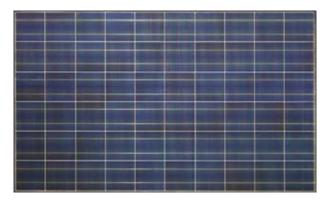
PV module (1592 mm x 962 mm) with an efficiency of 15.2% made from sixty solar cells. Using efficient module technologies, scientists at Fraunhofer ISE were able to reduce the losses in efficiency from the cell to the module level to only 5%.
