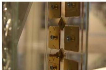
Even more concentration: The Fraunhofer ISE works on increasing the efficiency of CPV modules using e.g. secondary optics. ©Fraunhofer ISE
