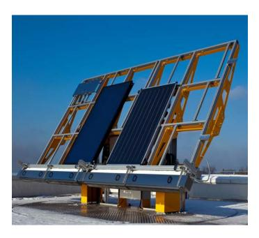
New precision tracker, developed in-house to characterize façade and large-area collectors as well as concentrating collectors. ©Fraunhofer ISE
