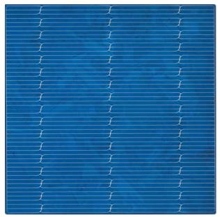
Photo: MWT solar cell of multicrystalline silicon (156 x 156 mm²). The Photo shows the contact structure with vias creating the contact to the back surface of the cell. ©Fraunhofer ISE
