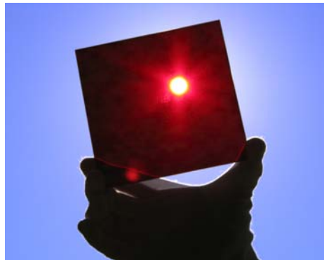
Light absorption of a glass plate coated with a thin amorphous silicon layer. ©Fraunhofer ISE
