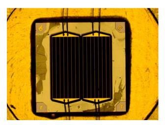
Figure 1: Photo of the new world record solar cell made of  $Ga_{0.35}In_{0.65}P/Ga_{0.83}In_{0.17}As/Ge$  with a cell area of 5.09 mm<sup>2</sup>.
