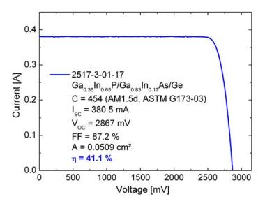
Figure 2: IV characteristics of the GalnP/GalnAs/Ge triple junction solar cell at a solar concentration of 454 suns. The measurements were carried out by the CalLab at Fraunhofer ISE.
