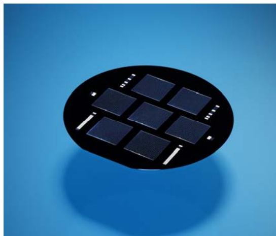
Four-inch wafers with seven highly efficient 4 cm 2 n-type silicon solar cells that reach efficiencies of up to 23.4%. Source: Fraunhofer ISE
